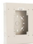
0608: Surface Mount Back Box. For use with FIRE ® RAY 50RU/100RU. Two 1/2"- 3/4" conduit knock-outs on each side. Universal back plate mounting with one conduit knock-out. Mounting holes for 0893 alignment bracket and 1000-020 wire cage.
